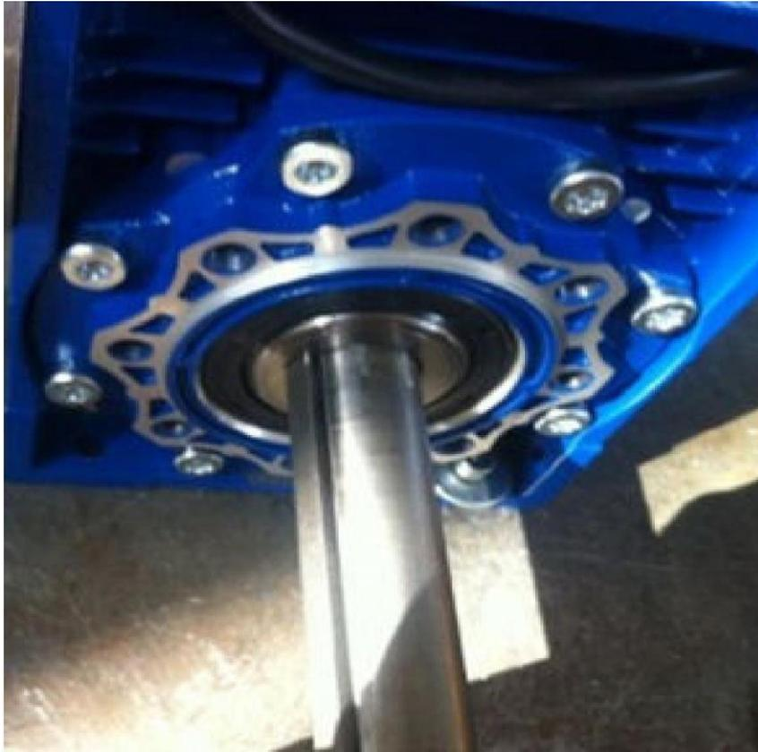
3. Insert the turning shaft on the required side and tighten the previously removed bolt
