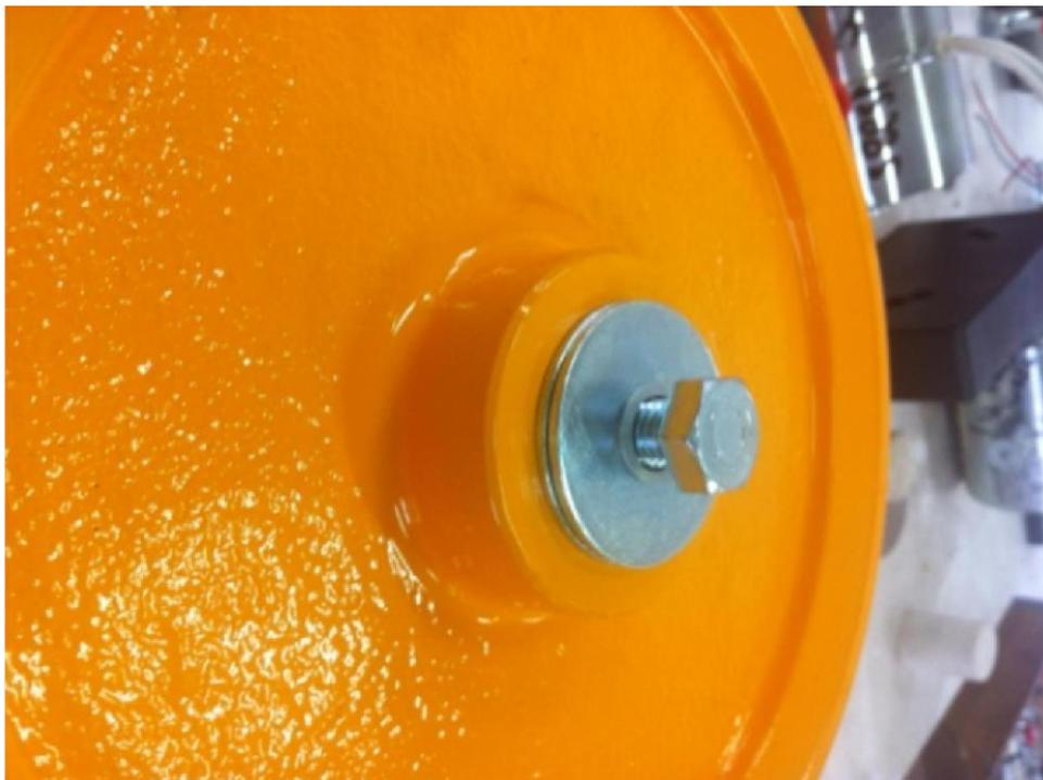
5. Re-insert the shaft with the pulley into the gearbox, on the required side
